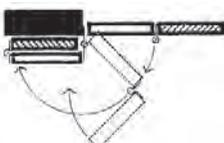
With folding action the centre window opens out over the outer window and the pair then swing 180° to park against the side wall.
